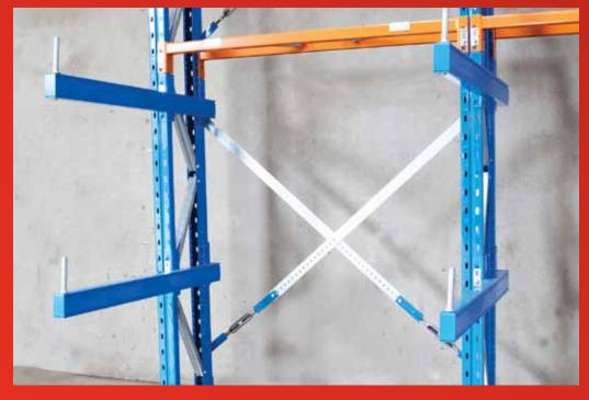
Turnbuckle spine bracing is used for lateral stability. This allows for re-adjustment of the structure should it be required. Frames are made up of two Keylock uprights and are joined together with bolted frame bracing to form a rigid column to support the cantilever arms.
