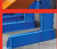
Columns are mounted to either single or double entry bases. Bases feature web stiffener plates at key points of concentrated stress. Heavy duty stud anchors provide secure floor fixing.
