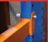
Arm locking pins are used to restrain the arm onto the column. A lynch pin is used as a safety lock to secure the arm and locking pin to the column.
